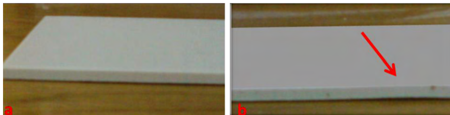
Fig. 8. Pictures of (a) the N1 and (b) the N4 porcelain stoneware tile samples after sintering at 1220 °C.
